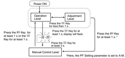
For details on the setting method, refer to 5-12 Performing Manual Control.
