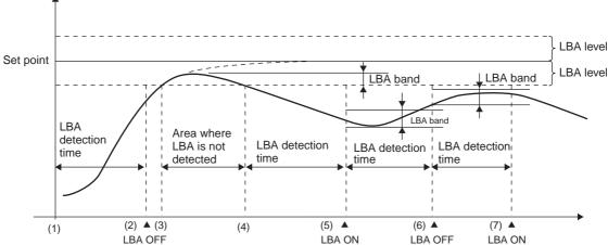
· Loop burnout alarms are detected at the following times.
