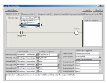
2. The Logic Operation Editor will be displayed. Confirm that the screen for work bit 1 is displayed, and select *Operation 3* from the *Operation Type* Field.
