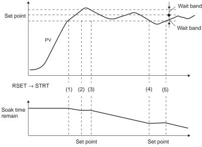
The wait band is the band within which the process value is stable in respect to the set point. The soak time is measured within the wait band. The timer that measures the soak time operates only when the process value is within the wait band around the set point (i.e., SP  $\pm$  wait band). In the above diagram, the timer will be stopped between the start and (1), (2) and (3), and (4) and (5) and will measure the time only between (1) and (2), (3) and (4), and (5) and the end.
