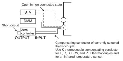
Disconnect the STV to enable the thermocouple of the cold junction compensator. When doing this, be sure to disconnect the wiring on the STV side.
