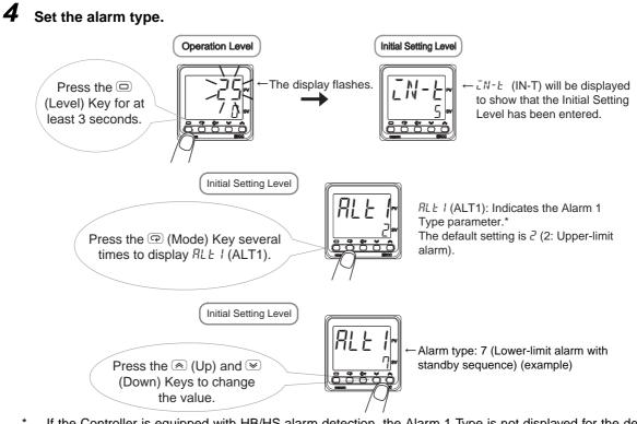
\* If the Controller is equipped with HB/HS alarm detection, the Alarm 1 Type is not displayed for the default settings. To use alarm 1, set an output assignment to alarm 1. For details, refer to 4-6-3 Assigned Output Functions (Assigning Control Outputs Is Not Supported for Position-proportional Models.).
