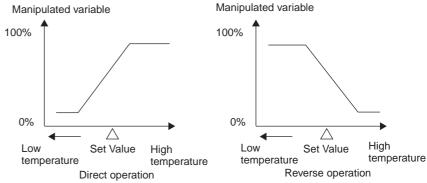
For example, when the process value (PV) is lower than the set point (SP) in a heating control system, the manipulated variable increases according to the difference between the PV and SP. Accordingly, reverse operation is used in a heating control system. Direct operation is used in a cooling control system, in which the operation is the opposite of a heating control system. The Control Output 1 Assignment is set to  $\bar{a}$  (control output (heating)) for either direct or reverse operation.
