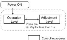
To move to the Adjustment Level from the Operation Level, press the
