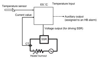
This alarm cannot be used for the cooling control output. With the default settings, the HB alarm is output on auxiliary output 1. You can use the output assignment parameters to change the output. You can use an integrated alarm to output an OR of alarms 1 to 4 and the other alarms. For details on the integrated alarm, refer to *5-9 OR Output of Alarms*.
