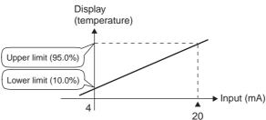
In this example scaling is set to display 4 to 20 mA as 10.0% to 95.0%.
