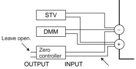
Compensating conductor of currently selected thermocouple. Use K thermocouple compensating conductor
