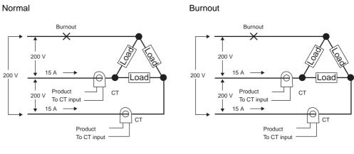
Current when there is a burnout =  $10 \text{ A} \times \sqrt{3} \times (\sqrt{3}/2) = 15 \text{ A}$
