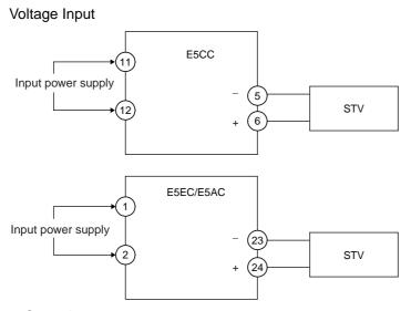
• Operation Set the STV output to the voltage or current test value.
