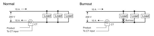
The heater power supply provides 15 A when the current is normal, and 10 A when there is a burnout, so the heater burnout detection current is calculated as follows:
