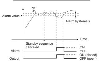
Alarm type: Lower-limit alarm with standby sequence
