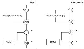
1. Connect a DMM to the transfer output terminals.
