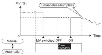
For a Position-proportional Model, the manual MV changes as shown below when there is a potentiometer input error.
