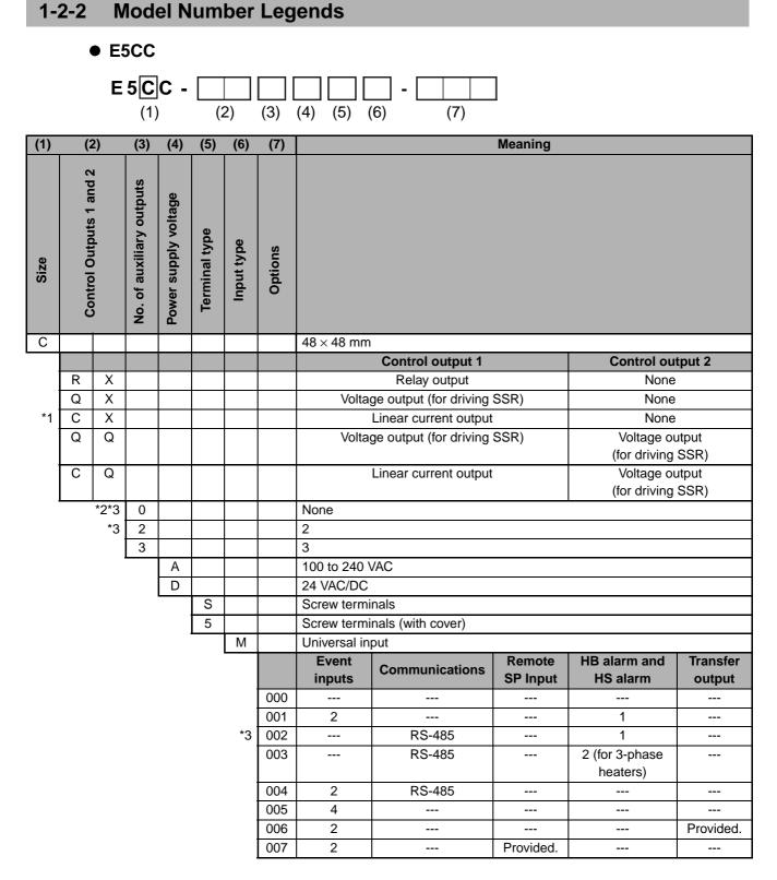
\*1 Options with HB and HS alarms (001 and 003) cannot be selected if a current output is selected for the control output. The control output cannot be used as a transfer output.
