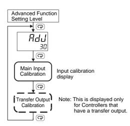
For Controllers that have a transfer output, the transfer output calibration display will be displayed after input calibration has been completed.
