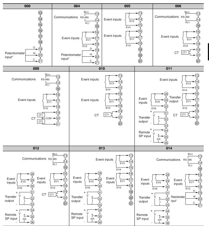
\* Can be used for a Position-proportional Model. These terminals are not used on other models.
