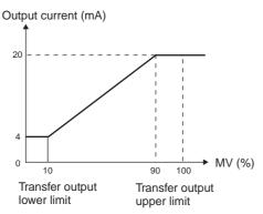
(The above graph is for when transfer output signal is set to 4 to 20 mA.)
