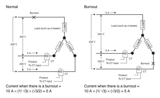
The heater burnout detection current for this connecting line is 5.4 A = (5.8 + 5) / 2.
