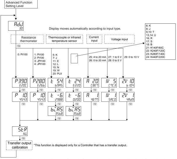
When calibration has been performed after purchase, the user calibration information shown in the following illustration will be displayed when moving to the Calibration Level.
